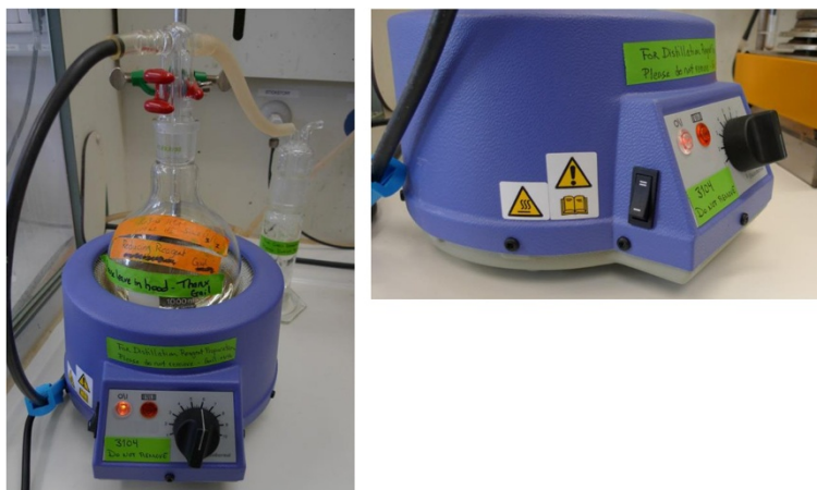
Figure 1 STRIP reagent preparation. The reagent preparation generates a lot of acid fumes, therefore the flask top must be firmly set and clamped in place and a gas wash flask attached to the outlet. With our set-up, we set the switch on the side to the “I” position and the dial to the 6 setting. The unit took approximately 30 minutes to bring the acid to a boil.
