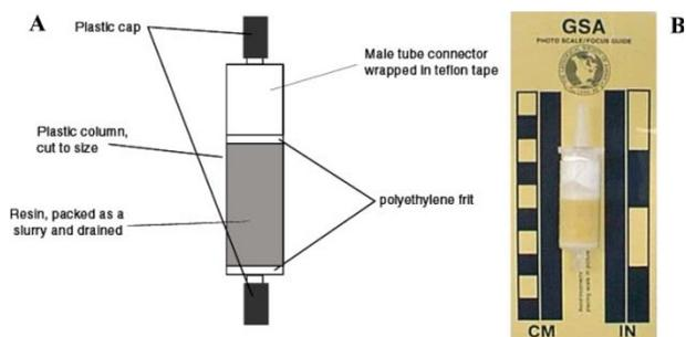
**Fig. 1** A: Schematic of resin column; B: picture.
