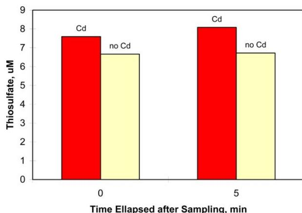
**Fig. 3** Effect of addition of Cd on thiosulfate concentration. Test conducted at Ojo Caliente, YNP. 0.5 mL 0.5 M Cd acetate was added to 60 mL sample. Analysis were conducted on site using a mobile lab parked next to the spring.
