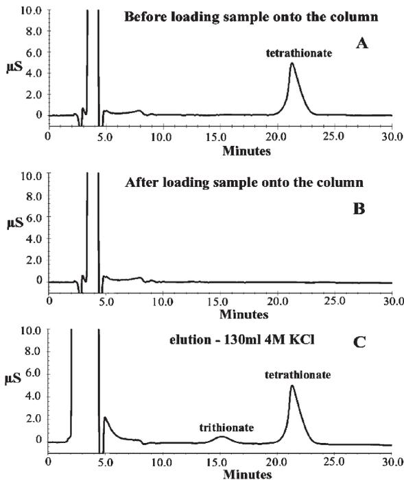
Fig. 5 Results of AG2-X8 resin elution with 4 M KCl elution.
