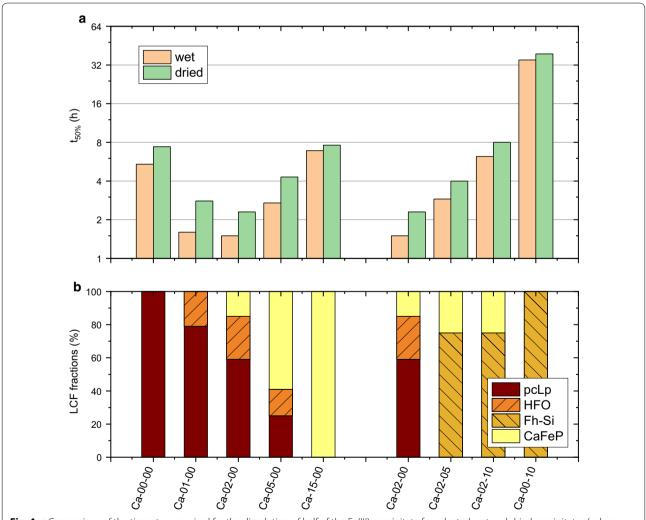
**Fig. 4** a Comparison of the times t<sub>50%</sub> required for the dissolution of half of the Fe(III)-precipitate for selected wet and dried precipitates (values from Table 2). **b** Structural information obtained by Fe K-edge EXAFS spectroscopy on dried precipitates (from Ref. [20]; *pcLp* poorly-crystalline lepidocrocite; *HFO* hydrous ferric oxide, *Fh-Si* silicate-containing ferrihydrite, *CaFeP* amorphous Ca–Fe(III)-phosphate)
